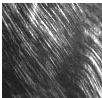
Figure 7. Polarized optical microscopy image of a 10% (w/w) solution of 2b in hexadecane. Magnification 100 \times .
